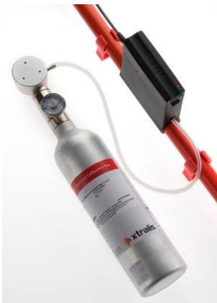
To verify gas sensors continue to respond to gas and that their accuracy is within acceptable limits; it is industry practice to regularly test / recalibrate all gas detectors (typically 6 monthly) using zero gas (e.g. nitrogen or air) plus the target gas of a known concentration (Typically 50% of full scale).
